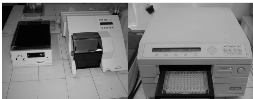
Linie ELISA BioRad (incubator, spalator si cititor)
